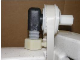
9. Turn retaining nut until it hits the bottom of the drive unit housing. (This adjustment may need to be tweaked once the drive unit is in place in the boat and while being used. Too loose or too tight will cause a ratcheting sound during pedaling. Tighten set screw to keep retaining nut in place.
