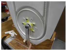
Turn crank and the belt will find its way onto the large sprocket.
