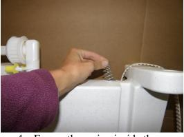
4. Ensure the spring inside the forward aluminum tube is still there
