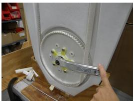
7. Put belt on crank side large sprocket and both small sprockets. Begin to thread on the idler large sprocket.
