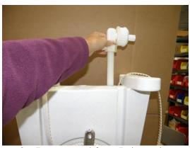
3. Remove rod from Drive unit housing
