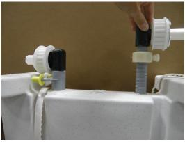
6. Replace with gray (fiberglass) threaded rods and small sprocket assemblies.
